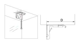
For Top Standar Rail: Attach the rail in the front edge of the clip and push the back of the rail upwards (till it clicks in) as below drawing
